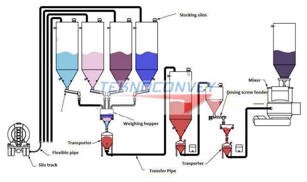
Applications of dense phase conveying vessel:
